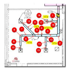
What is not shown but you should always include are volume dampers at each individual branch connection to an air distribution device. This allows for the adjustment of airflow.
